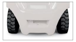
**Designed for Durability** The one piece casting and floating design of the drive axle allows for the shock of operation to be absorbed by the housing rather than the axle itself, increasing, longevity and durability.
